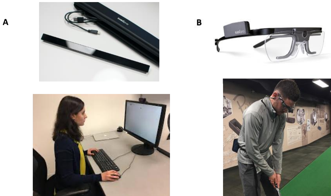
Figure 2. Images of the fixed (left) and wearable (right) eye trackers used in the School of Psychology. The eye tracker in panel A is the Tobii X3 120. In the lower panel, the X3 120 is attached to the bottom of the computer monitor as a participant performs a task. Panel B depicts the Tobii Glasses 2; in the lower panel, a participant wears the glasses while practicing golf.
