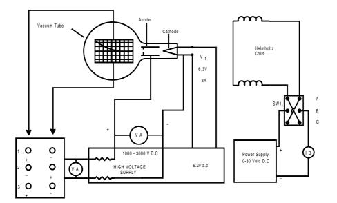
Figure 11.1: The circuit diagram for the e/m apparatus.
