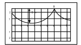
Figure 11.3: Trochoid trajectory of the electron beam using the electron mirror set-up.
