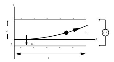
Figure 11.2: Trajectory of an electron passing between two charged plates of length L.
